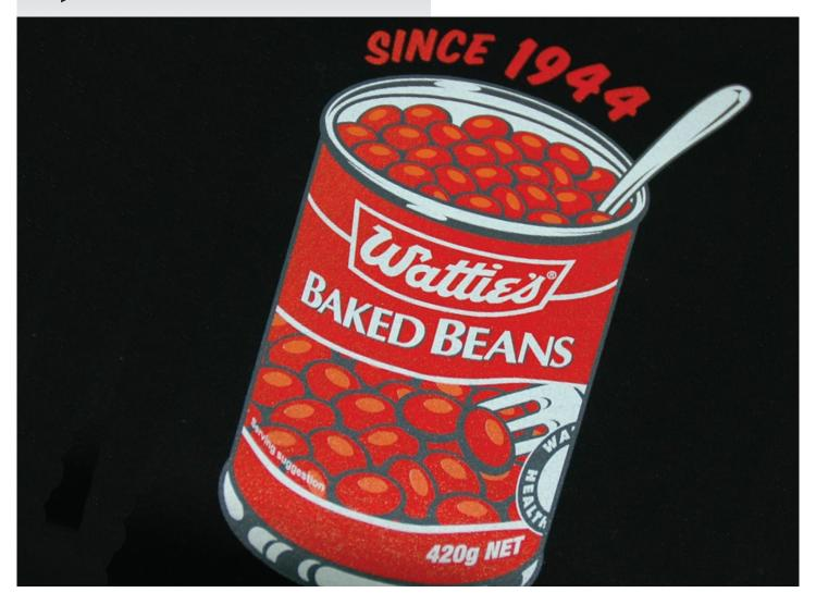
This is the most common of screen prints. Art is separated into the different colours and a screen is made for each. With a dark shirt a white base print is put down and the colours go on top of this. It is a little more expensive than printing on a white shirt as each colour needs to be cured before the next colour goes on.
